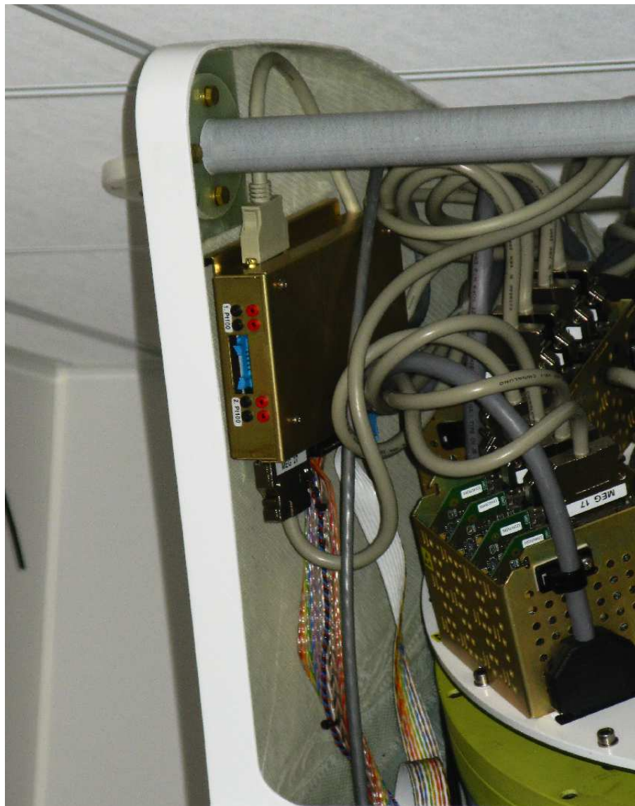
Figure B.1 He level meter board (with covers on) inside the gantry
