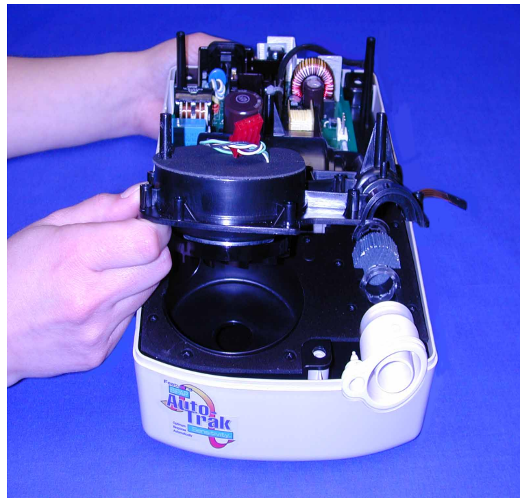
Figure 6-23 Removing the Blower Assembly
