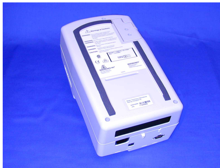
Figure 6-4 Removing the Bottom Enclosure Screws
