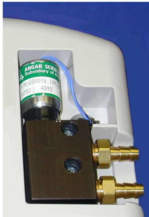
Figure 8-2 Removing the Oxygen Module
