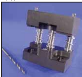
Tappet Guide Puller Tool for 1957-85 Sportster, replaces 95724-57. VT No. 16-0157
