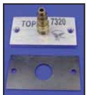
Front Low Pressure Master Cylinder Bleeder Covers will allow one person to bleed brake lines or to check system for leaks and can drain the entire system to replace brake fluid.
