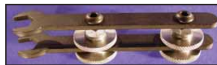
Sifton Pushrod Adjusting Wrench eliminates the need for 3 hands, dual wrench holds 2 outer nuts. The inner is tightened with a separate wrench, fits 7/16" hex nuts and is fully adjustable for solid lifters. VT No. 16-0819
