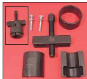
Jims Cam Assembly Tool for all 2006-up Dyna and 2007-up FXST, FLT models. Used to hold both cams in an upright position while lowering the cam support plate over cam journal. VT No. 16-0323
