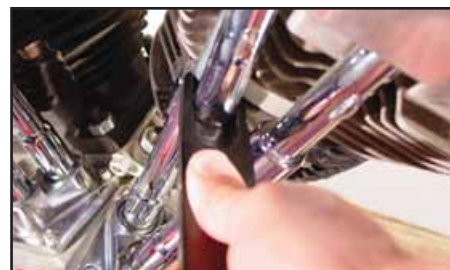
Sifton Pushrod Adjustment Gauge for use on Big Twins 1953-84 with hydraulic lifter. Replaces 91438-79. Complete with instructions. VT No. 16-0993
