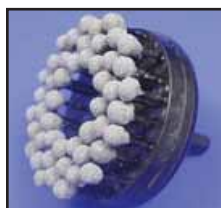
Flex Hone for Rotor designed to produce a swirl or cross hatch pattern with a non-directional finish which reduces friction induced braking noise: medium grit. Designed for low speed operation using a 3/8" drill. Available for Master Cylinder Bore.
