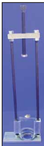
Shock Absorber Tool. Replaces 97010-52A to simplify shock absorber disassembly or assembly by holding spring in compression while disassembling parts. Includes 97019-52A block.
