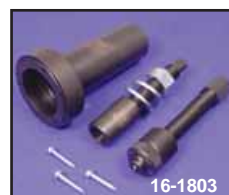
Big Twin Mainshaft Seal Remover & Installer replaces 95660-42. Use to install and remove main seal. This tool will push seal in as flat and straight as possible to .050 below housing for a no leak fit.
