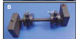
Shifter Fork Gauge is used to set and align shifter forks on Big Twin 4-speed models.
