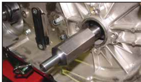
4-Speed Transmission Arbor replaces clutch hub nut to allow test rotation with 1/2" drill. VT No. 16-1274
