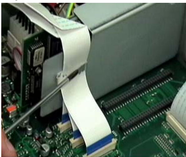
Remove the two screw that hold the modem in
