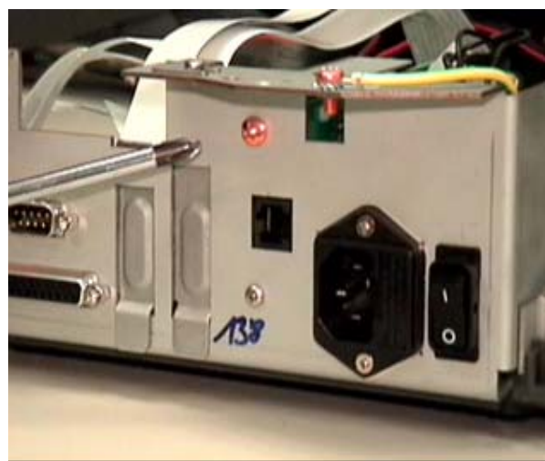
Remove the two screw that hold the modem in
