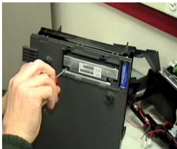
Loosen the two torx screws on the PSD
