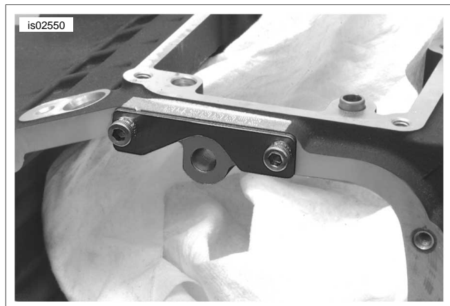
Figure 1. Install Drill Plate to Transmission Case
