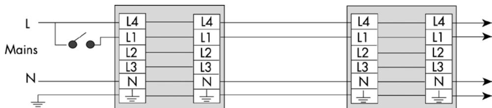
**Connection of MAX HF in series, with a double pole switch**
