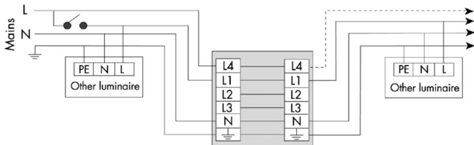
**Connection of MAX HF-E in series with other luminaires, with a double pole switch**
