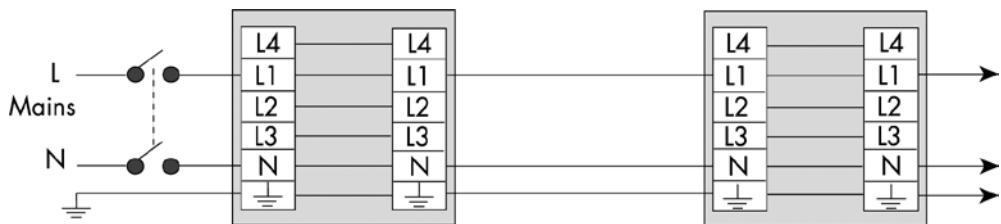
**Connection of MAX HF-E in series with other luminaires, with a single pole switch**
