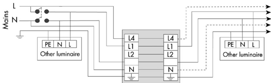
**Parallel connection of MAX HF-E with other luminaires and a double pole switch**
