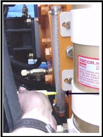
Figure 2-3: D2P oil level—engine not running
