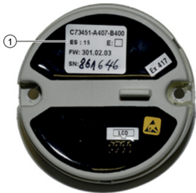
Example of application electronics for SITRANS P DS III with PA and FF
