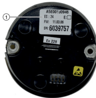
Example of application electronics for SITRANS P DS III with HART
