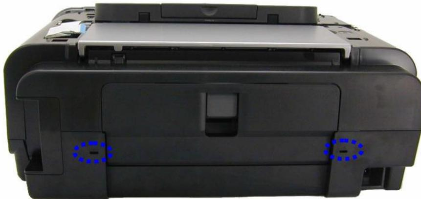
(V) Release the hook on the left side of the printer, then while inserting the flat-blade screwdriver in the slots on the left and right sides of the printer front, release the hooks to remove the main case from the bottom case.
