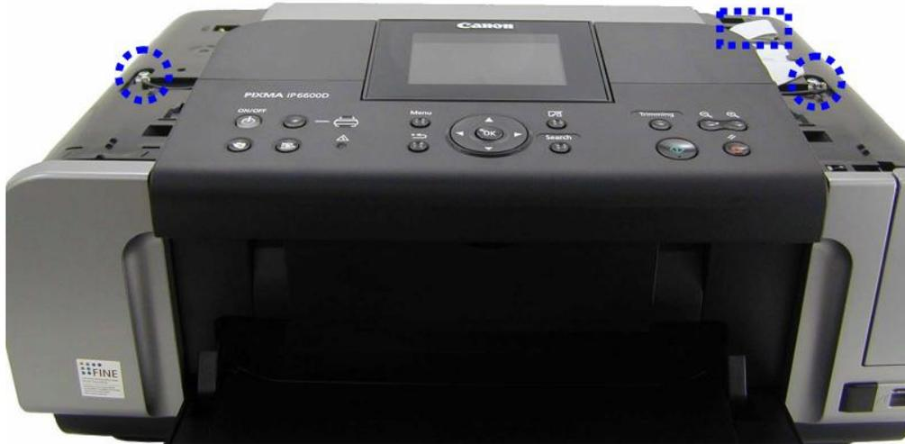
(III) Release the hooks and remove the front left cover as shown below.
