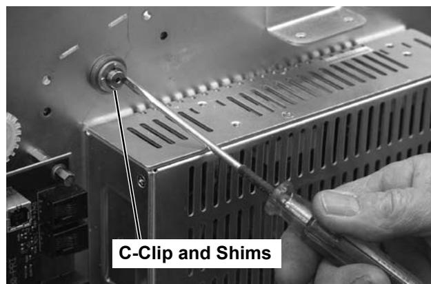
Figure 6-12 Remove C-Clip and Shims
