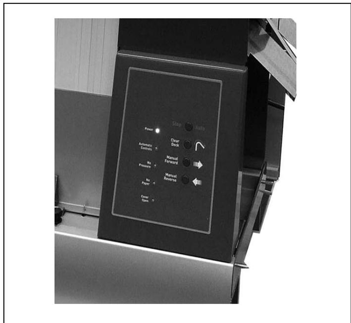
**Figure 4-4** F734/F735 Control Panel Overlay
