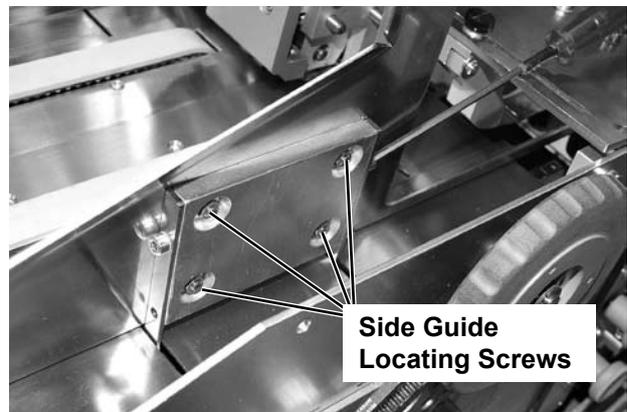
Figure 6-4 Material Side Guide Screws
