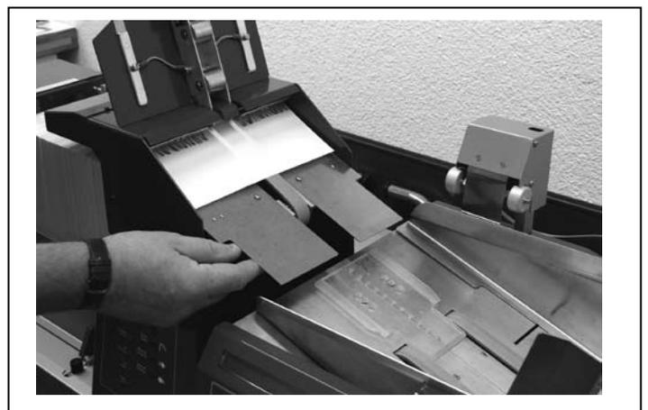
**Figure 4-7 Lift F734/F735 Exit Deck**
