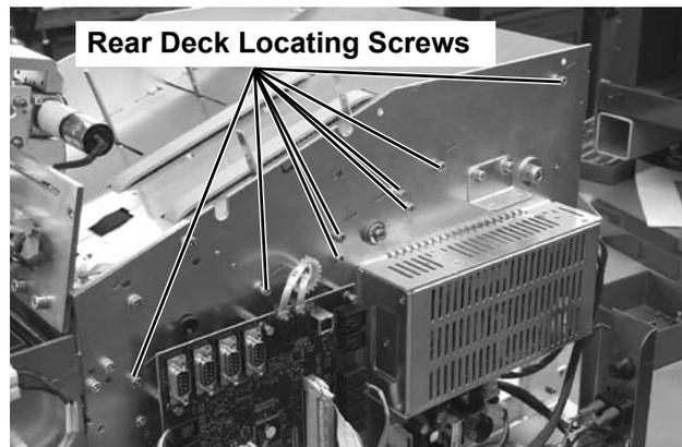
Figure 6-11 Remove Rear Deck Locating Screws
