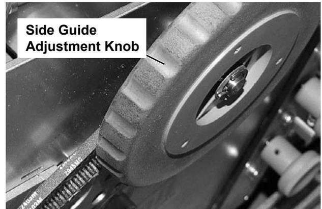
Figure 6-7 Remove Knob, Pulley and Belt
