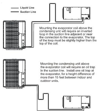
Insulation is necessary to prevent condensation from forming and dropping from the suction line. Armflex (or satisfactory equivalent) with 3/8" min. wall thickness is recommended. In severe conditions (hot, high humidity areas) 1/2" insulation may be required. Insulation must be installed in a manner which protects tubing from damage and contamination.
