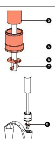
Pull the extractor rod so that the upper face of the washer stops against the lower face of the guide bush. Insert the aluminium bush (A) in the seat of the sealing ring.
