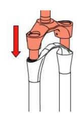
In a graduated recipient, prepare the quantity of oil to pour into the fork leg (see table). Pour roughly 1/3 of the oil required into each stanchion, then pump the fork a few times to eliminate any
