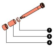
Insert the bushing in the piston rod through the hole with smaller diameter. Insert the pumping element (3) into the stanchion.
