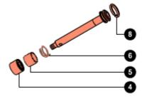
If the piston segment (8) is damaged, you can prize it off with a small flat-tip screwdriver.
