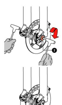
With a 4mm Allen wrench, tighten the screws (3) on both dropouts to the recommended tightening torque (6 Nm  $\pm$  1).
