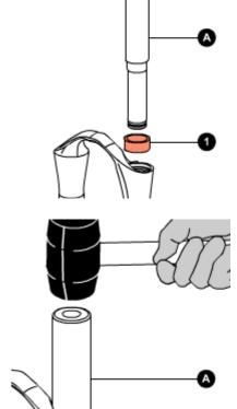
Using a hammer knock the introducer (A) into the arch-slider assembly.
