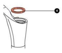
Smear the dust seal and the sealing ring with some grease.
