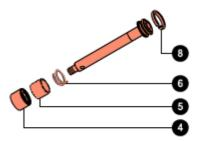
Insert the pre-assembled valve in the piston rod from the three-point ring side as shown. Insert the valve and the pumping element (3) into the stanchion.
