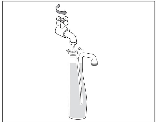
Fig. 13 Filling the condensate trap with water
