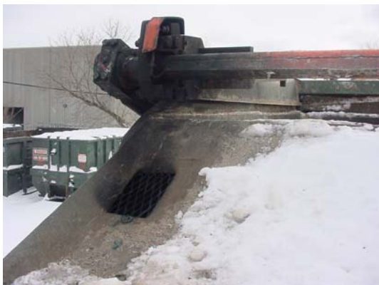
Figure 6-D: Existing condition of exhaust gases blowing back directly on the fork.
