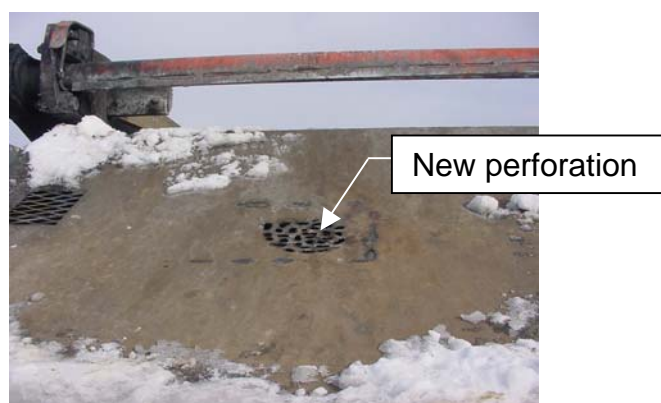
Figure 6-G: Cab guard modification so the exhaust gases are exiting in the center of the cab guard, between the forks. In this example, a welding torch was used to create a perforated exhaust exit in the cab guard.
