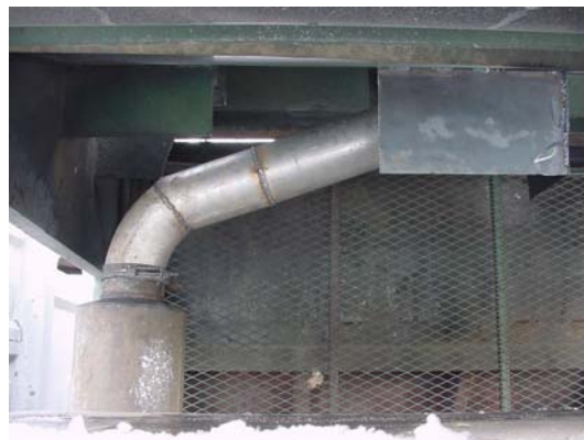
Figure 6-E: View under the cab guard showing the rerouted exhaust pipe to the center of cab guard.
