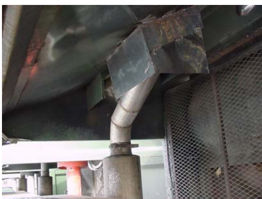
Figure 6-F: View under the cab guard showing the rerouted exhaust pipe.
