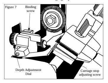
be a high point on the cutter; the adjustment should be made to the high point. If the cutter does not touch the key blank after one rotation, proceed to change the adjustment.
