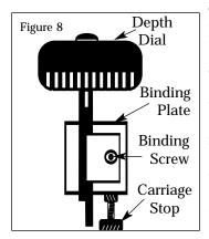
To adjust the cutter guide, loosen the binding screw on top of the cutter guide **slightly**. (see Fig. 7 & 8). Once you have loosened this screw, the depth adjustment dial can be rotated to the left (to decrease depth of cut) or to the right (to increase depth of cut). Again, proper adjustment will be achieved when the cutter
