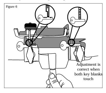
To check the depth adjustment, insert two identical key blanks into the vise jaws, setting them flat in each vise. (It is not necessary to align the blanks.) Then, raise the carriage, positioning the left blank against the cutter guide and the right blank against the cutter. Next, turn the machine pulley by hand and note the right key blank. The cutter should just barely graze the key blank when the adjustment is correct.
