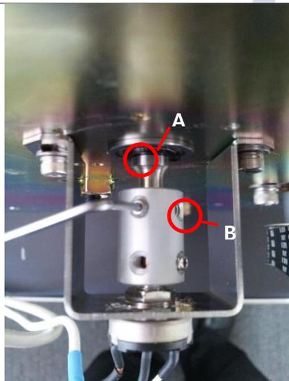
Unfasten the 2 set screws using a hexagonal wrench (hexagonal wrench: 1.5").
