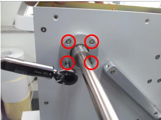
Unfasten the 4 set screws using a hexagonal wrench (hexagonal wrench: 3").
