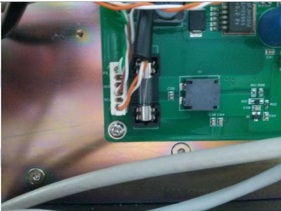
Open the rear case on the underside to find the control PBA. The 3A fuse is on the bottom left corner of the control PBA.
