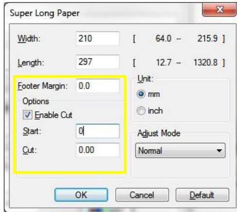
6. Set the Adjust Mode as the No Adjustment when using regular roll media.
