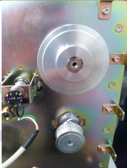
When the 2 screws are unfastened as above, the unwind motor can move up and down. Unfasten the belt slightly lifting the unwind motor.
