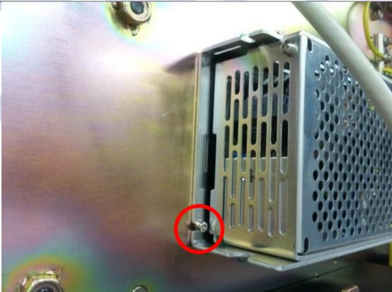
The fuse is fixed by two cross recess bolts. First, unfasten the bolt on the bottom left corner.
