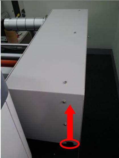
After loosening the bolts, lift up by inserting fingers inside the circle marked with red.
