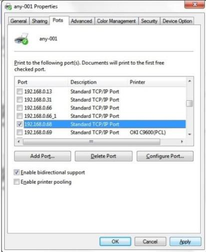
If the port does not corresponds to the one used, click the relevant port being used and click the APPLY button and then the CONFIRM button.
