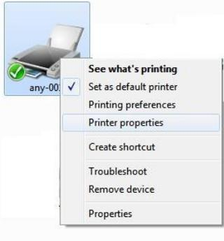
Select [Printer properties] or [properties] by clicking the right button of the mouse on Any-001 Printer.
