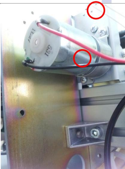
Cutter can be disassembled only after removing the cutter motor. Disassemble the cutter motor after unfastening the screws in the red circles.
