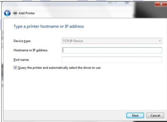
After entering a printer's IP address, click [Next]. (Refer to 2.2.3.1 How to check IP Address to check the printer's IP.)
