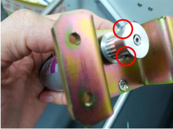
Unfasten the two set screws of the feed motor pulley using a hexagonal wrench (hexagonal wrench: 2")
