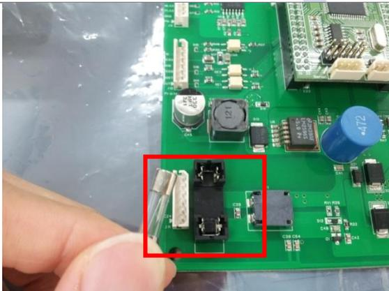
When needed, the fuse of the control board can be replaced in the way shown above.
