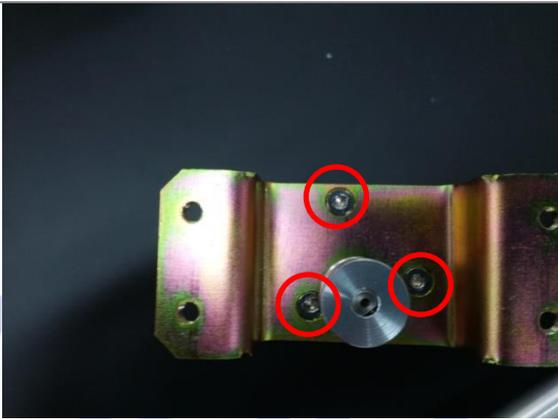
Disassemble the feed motor and the bracket using a hexagonal wrench (hexagonal wrench: 2.5")
