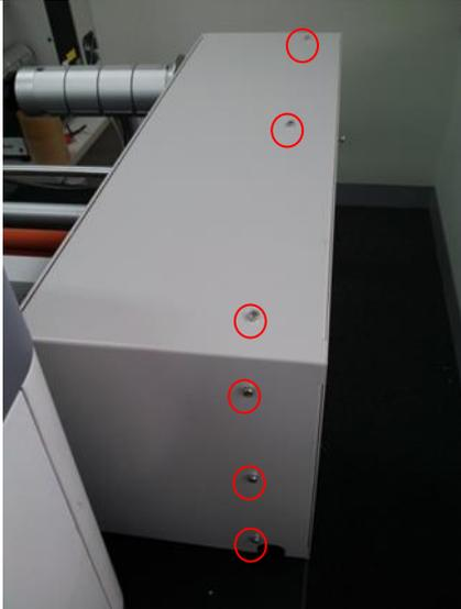
Open the rear cover of the press station using a hexagonal wrench (hexagonal wrench: 2.5", 3").
