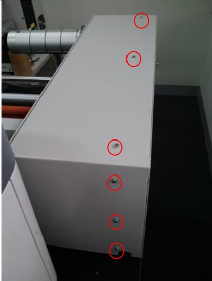
Open the top cover of the press station using a hexagonal wrench (hexagonal wrench: 2.5", 3").
