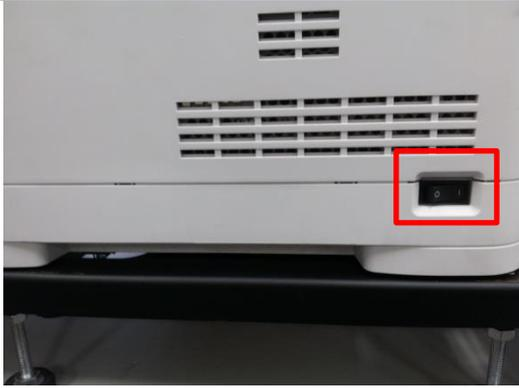
Turn on the digital printer power by pressing the POWER button.
