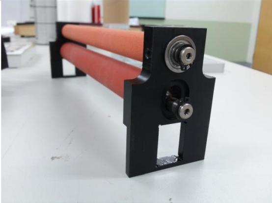
The figure shows the feeding roller after it is removed.
