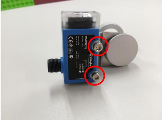
Unfasten the screws in the red circles using a hexagonal wrench (hexagonal wrench: 3").
