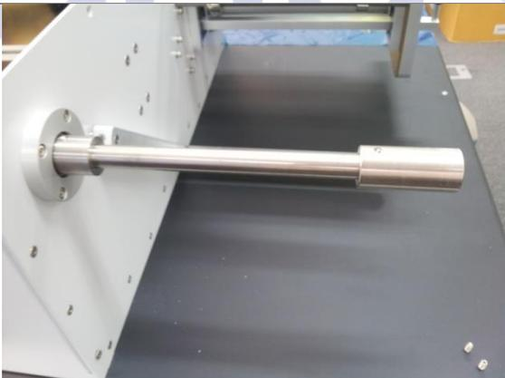
When the bobbin is slowly pulled out by hand after unfastening the two set screws, the part shown in the figure comes out.
