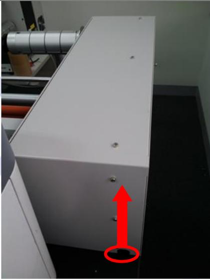
After loosening out bolts, lift up by inserting fingers inside the circle marked with red.
