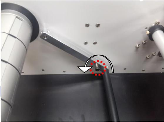
Loosen the fixing bolts fastened to the left and right tension bars of the any-001 by turning them counterclockwise.
