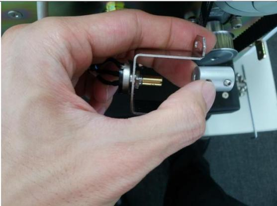
The potentiometer can be pulled out holding the sleeve by hand.
