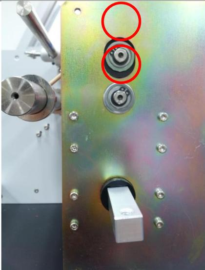
A close-up photograph of a vertical metal plate with a rainbow-like finish. Two circular rings are mounted on the plate, one above the other. Both rings are circled in red. To the left, a portion of a mechanical assembly is visible. Below the rings, there is a white rectangular component partially inserted into a slot. | <p>Unfasten the rings using a ring remover.</p>                                                                           |
