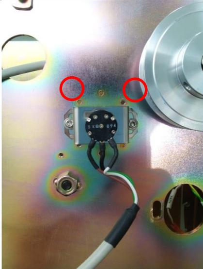
Remove the fixed bracket of the potentiometer by unfastening the 2 screws using a hexagonal wrench (hexagonal wrench: 2.5").
