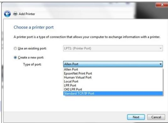
Select [Create a new port], then from the drop-down Allen Port menu, select [Standard TCP/IP Port] and click [Next] when using LAN.
