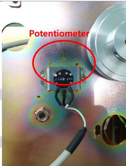
When the rear cover of the press station is opened, you can see the potentiometer installed as shown in the figure.
