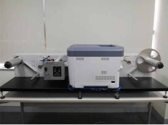
A photograph showing a white and blue printer station with a blue top, mounted on a black table. The station is positioned between two large rollers. The printer is on the right side of the station. | <p>Put the any-001 press station on the table.<br/>(the weight of station is about 84 kg(185lbs), and printer is about 30kg(62lbs). Four people are required to lift the any-001)</p> |
