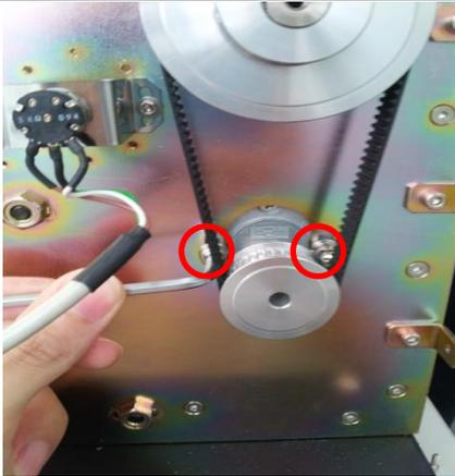
Unfasten the 2 screws using a hexagonal wrench (hexagonal wrench: 4").
