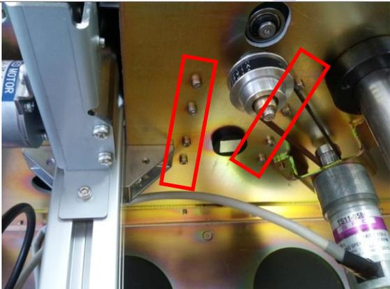
A close-up photograph of a mechanical assembly. A slide guide is being worked on. Eight screws are highlighted with red rectangles, indicating they need to be removed. The assembly includes a motor, a slide guide, and various metal components.                                                                            | <p>Remove the slide guide by unfastening the 8 screws at the back using a hexagonal wrench in the way shown in No. 2.</p> |
