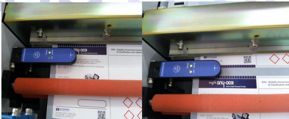
At this time, if the LED light of the sensor comes on above the black mark or a gap, it means that the setting has been normally completed, which can be also checked by the MARK LED light on the panel at the front of the equipment.
