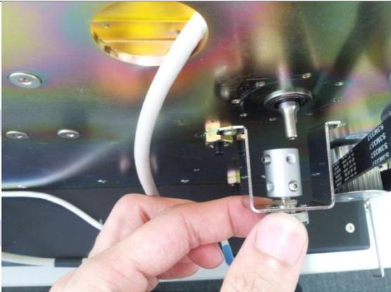
The potentiometer can be easily pulled out by hand.
