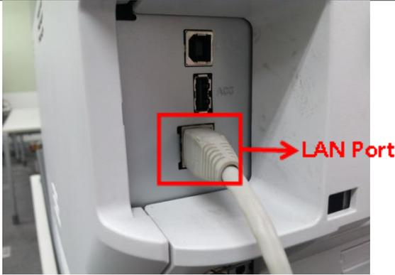
Turn on the printer power and connect the LAN cable to the LAN port. The other ends of the cable connect to the PC.
