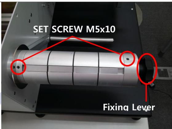
Unfasten the fixing lever of the unwinder by turning it counterclockwise. Then, unfasten the two set screws using a hexagonal wrench (hexagonal wrench: 2.5").
