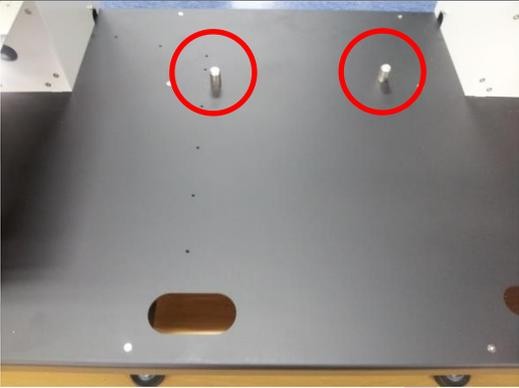
A close-up photograph of the top surface of the station. Two small, cylindrical metal protrusions are highlighted with red circles. These are the fixing bars mentioned in the text.                  | <p>Check the locations of two fixing bars of the station.</p>                                                                                                                         |
