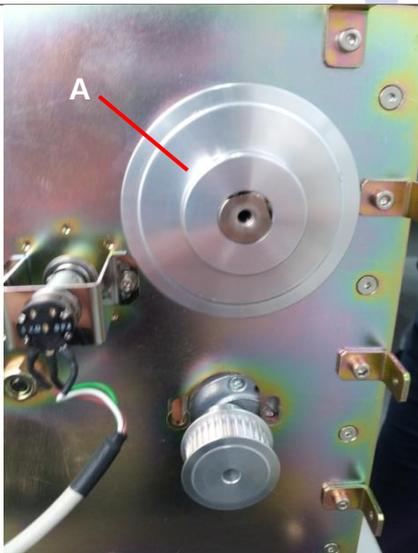
When the 2 set screws are unfastened as shown in No. 6, the unwindmotor can be moved up and down. Slightly lift up the unwindmotor and unfasten the Belt.
