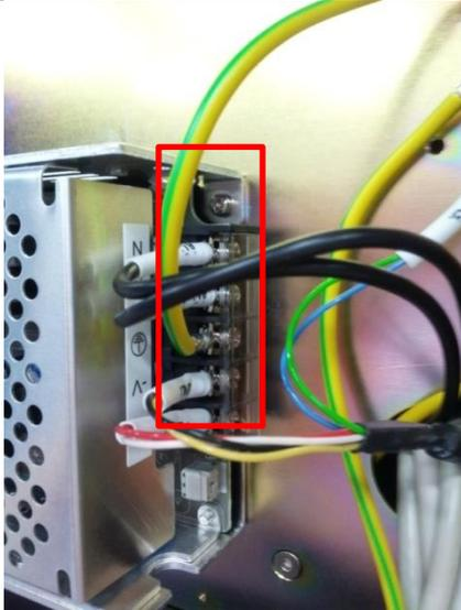
Unfasten the cable connected to each terminal using a phillips screwdriver.
