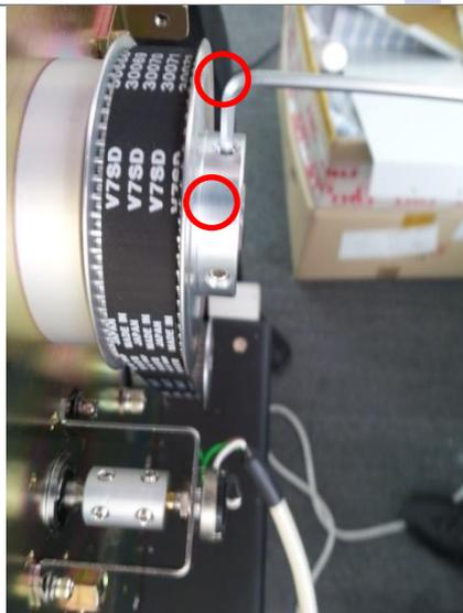
Unfasten the 2 set screws using a hexagonal wrench (hexagonal wrench: 2.5").
