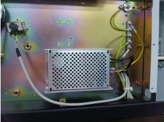
Open the rear case on the rewinder side to find the SMPS.
