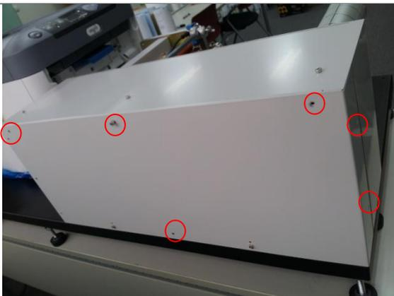
Open the rear cover of the press station using a hexagonal wrench (hexagonal wrench: 3").
