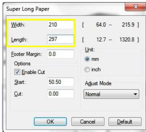
5. Footer Margin is a space between printed units, Start is a beginning point of images, and Cut is a cutting point after finishing all works.
