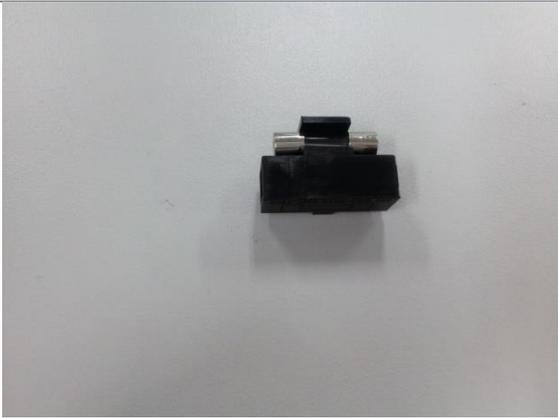
The fuse can be replaced in the way shown above (Fuse: 3A).
