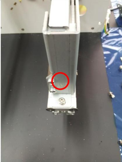
Unfasten the screws in front of the cutter using a hexagonal wrench (hexagonal wrench: 3").
