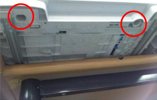
A close-up photograph of the bottom surface of the printer. Two circular holes are highlighted with red circles. These are the mounting holes used to secure the printer to the station.             | <p>These are two holes at the bottom surface of the printer are used to fix the printer to the station.</p>                                                                           |
