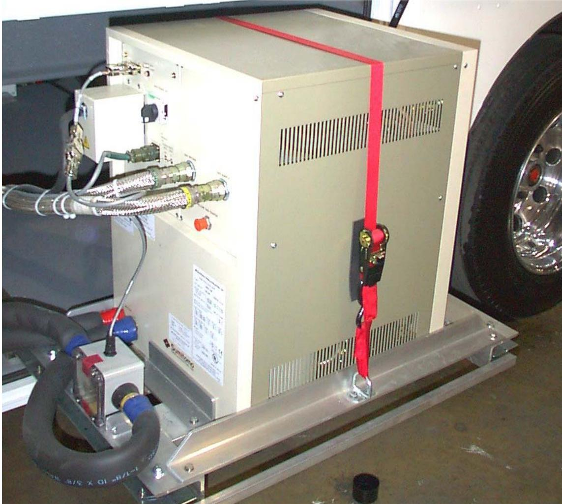
**Figure 5: Cryogen Compressor**
