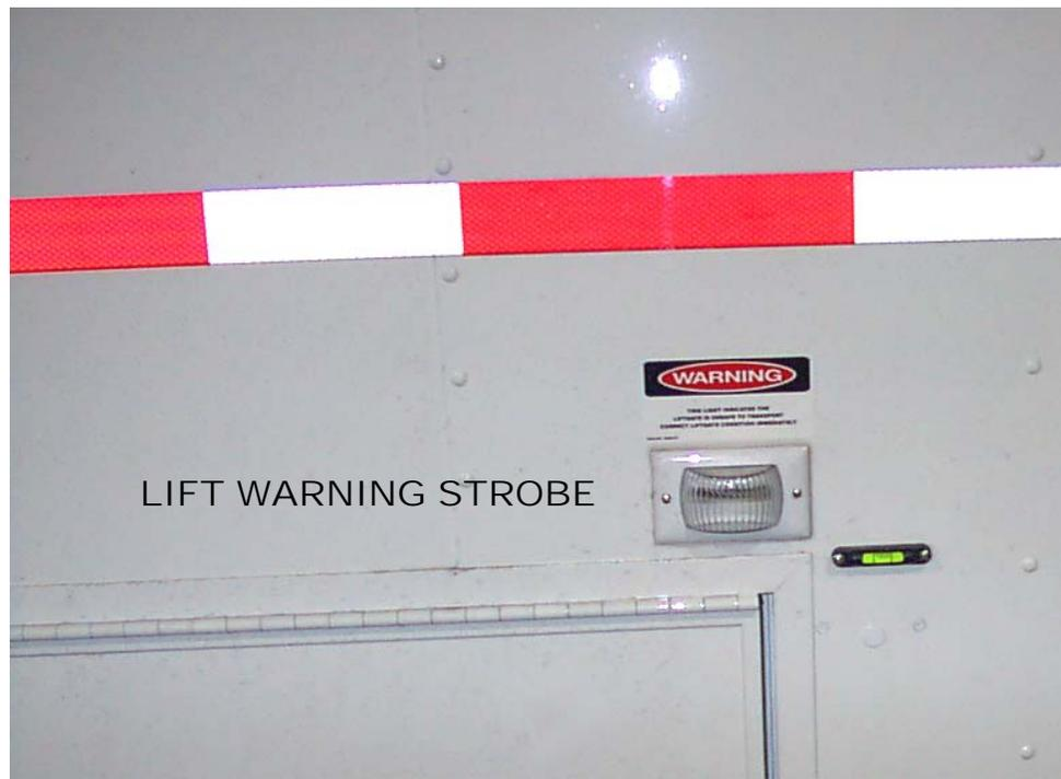
**Figure 63: Lift Transport Warning Strobe**
