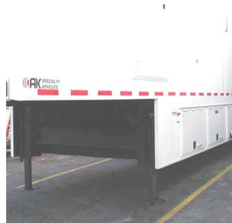
**Figure 51: Landing / Stabilizing Leg Assembly**
