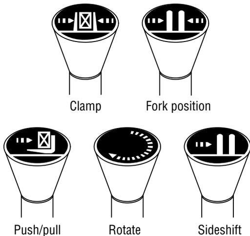
**Figure 3-5 Operator controls**
