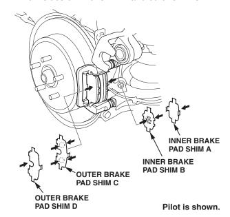
3. Install the new brake pad shims (four per side) on each rear caliper. For Pilots, refer to the 2003-04 Pilot Service Manual, page 19-19. For Odysseys, refer to the 1999-04 Odyssey Service Manual, page 19-26.
