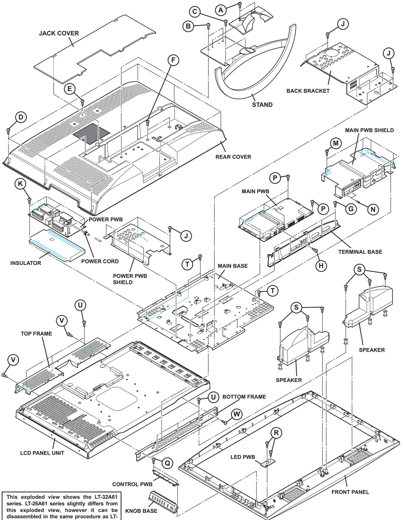
This exploded view shows the LT-32A61 series. LT-26A61 series slightly differs from this exploded view, however it can be disassembled in the same procedure as LT-26X506.
