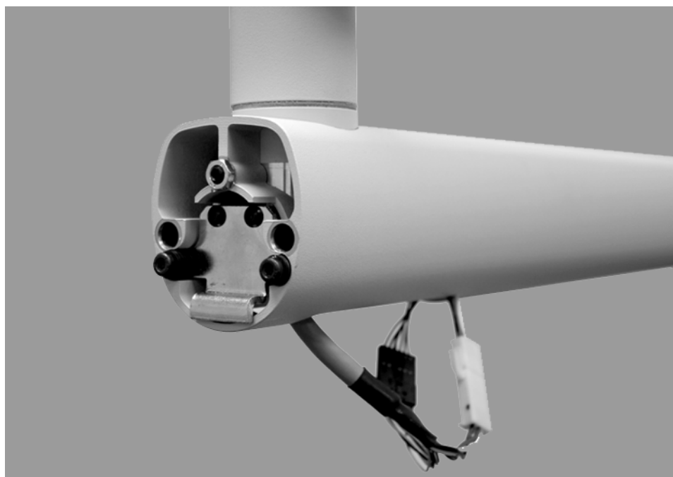
Figure 22 Connecting the Articulating Arm and Horizontal Arm Cables
