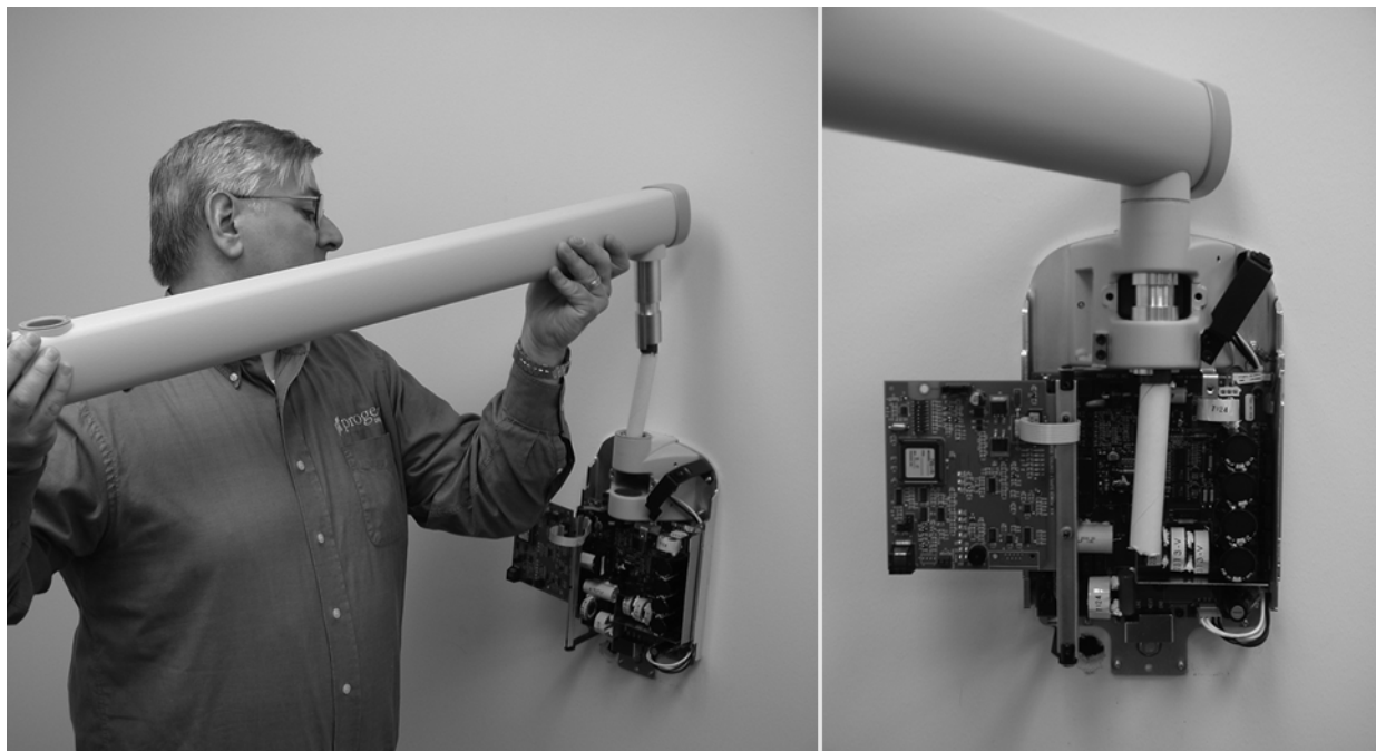
Figure 17 Installing the Horizontal Arm
