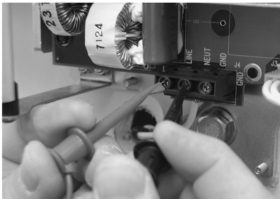
Figure 25 Verifying Input Voltage at the Line Input
