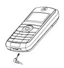
New batteries are shipped partially charged. Before you can use your phone, install and charge the battery as described below. Some batteries perform best after several full charge/discharge cycles.
