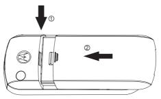
To prevent damage to the battery door, install only as described here.
