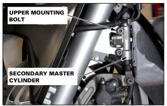
5. Loosen the lower secondary master cylinder mounting bolt by 90 degrees only.
