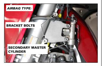
3B. Airbag type only; for all other types go to Step 4: Grasp the secondary master cylinder with one hand as shown and firmly rotate the cylinder and bracket in a clockwise direction.
