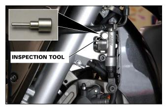
7. Grasp the secondary master cylinder with one hand as shown and firmly rotate the cylinder in a *clockwise* direction.
