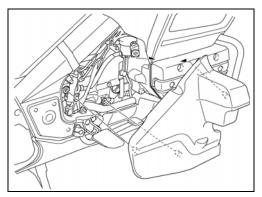
Apply a punch mark to the right frame spar, just above the rear master cylinder reservoir. See the following photo for placement.
