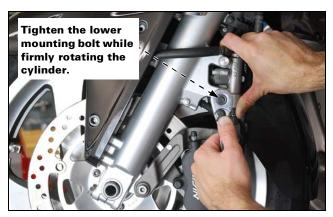
9. Grasp the inspection tool and check the tension by pulling lightly on the tool as shown. The tool should not slip out.
