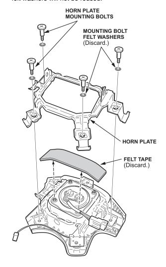
4. Remove and discard the felt tape covering the lower two inflator locknuts.
