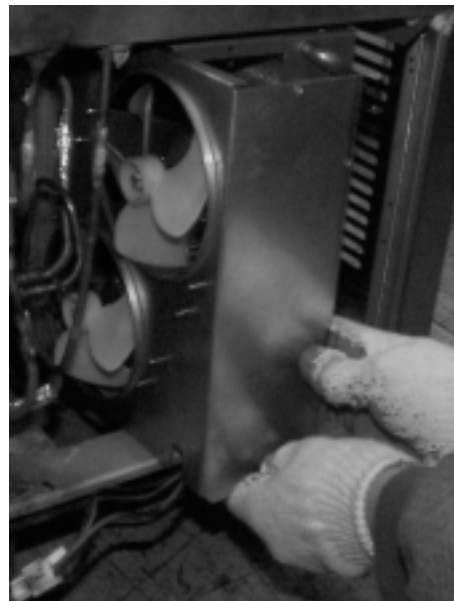
PULL OUT C-FAN MOTOR ASSEMBLY
