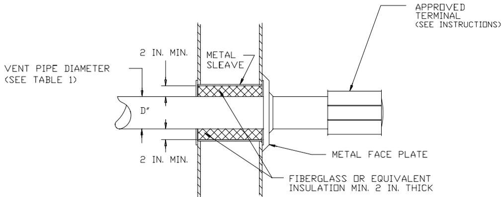
NOTE: DO NOT TERMINATE HORIZONTAL VENT WHERE CONDENSATE COULD CREATE A NUISANCE OR HAZARD OR COULD CAUSE BUILDING OR EQUIPMENT DAMAGE.
