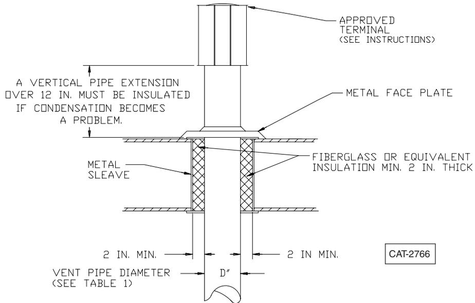
**Figure 10A. Horizontal Vent Installation**
