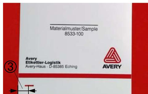
[2] Punch position = distance of punch center from (inner) edge of material (3).
