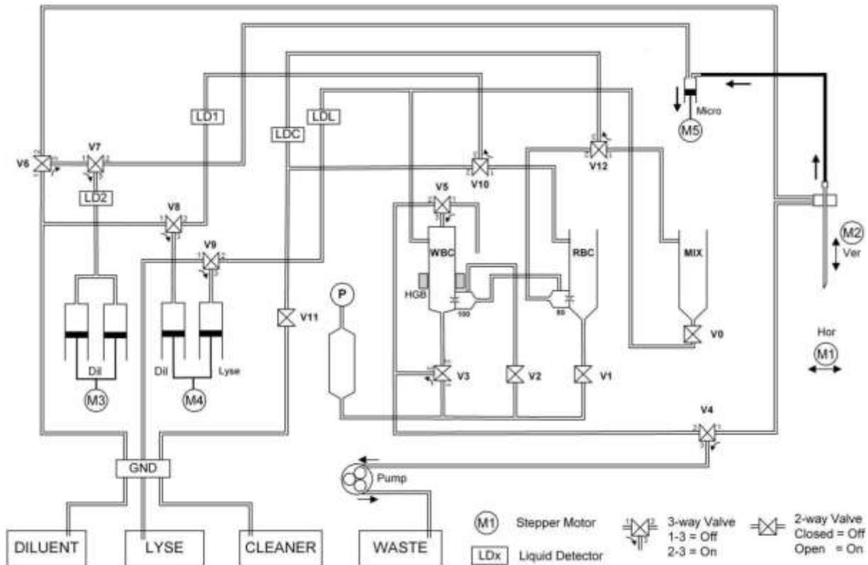
There is another sampling process for the second (RBC) dilution, when 35  $\mu\text{l}$  of primary dilution is aspirated from the MIX by the aspirating needle. Both of the samples are separated from the diluent with a small air bubble and there is another air bubble between the sample and the end of the needle.
