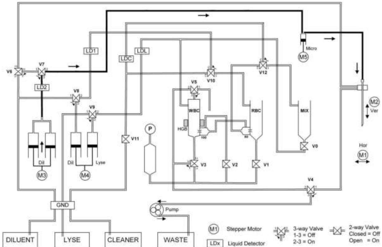
The second sampling process aspirates 35  $\mu$ l of primary dilution and then it is added with 4.0 ml of diluent (1.0 ml + 3.0 ml) into the RBC chamber. This process makes 1:18285 dilution rate in the RBC chamber.
