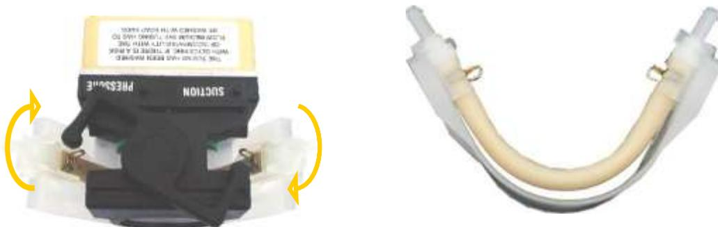
In case of damaged tubes, it can be replaced by a new one by opening the two metal locks located at the two ends of the tube (see picture).
