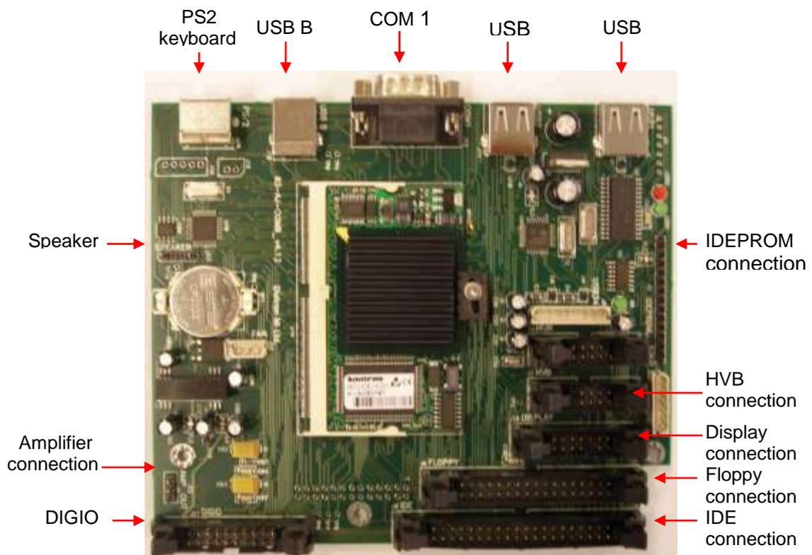
**PC system** of the COMB board is based on the DIMM-PC module, which is a credit card size PC with AMD Elan SC520 133 MHz micro-controller. DIMM-PC itself contains 16 or 32Mbyte RAM and same size of FlashDisk that acts like a hard disk. DIMM-PC module is easily replaceable as it has an open socket (it has also a screw for safe fixing). COMB card contains single ICs and some drivers/protection-circuits for the interfaces such as COM1, PS2, USB, IDE and Speaker.
