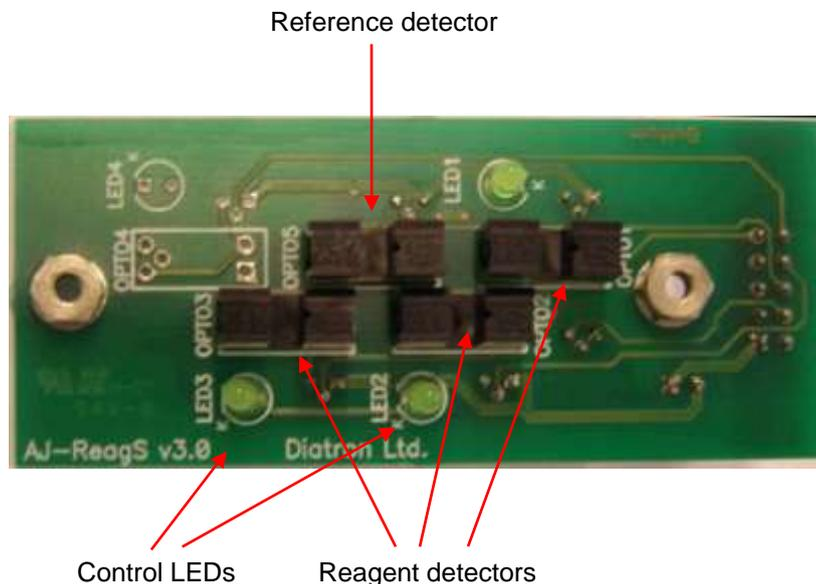
The Reagent Sensor Board is connected to the PPB card, and the valve driver micro-controller makes the sensing and compensating operations.
