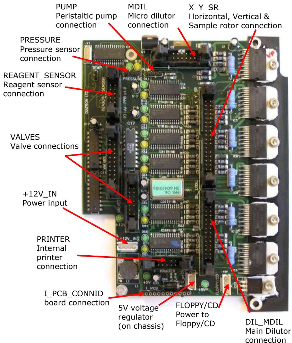
**PPB** card contains the main power regulator circuits, valve and motor driver circuits and other connections for the fluidic and pneumatic system's parts.
