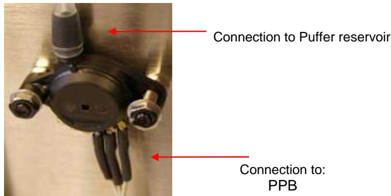
The pressure sensor can operate from +5V only. It is a calibrated sensor with 0-1.1 Bar input range. Do not apply more than 1.5 Bar to it, because it can ruin the pressure sensor.
