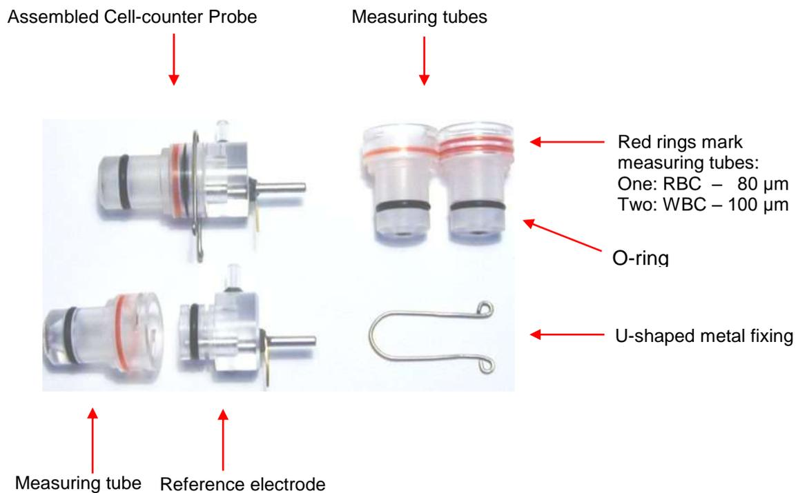
The aperture is made of ruby and it is moulded into the measuring tube.
