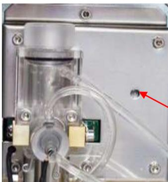
1. Locate the opening for offset setting potentiometer on the measuring block (see enclosed picture).
