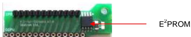
Keeping the hardware identity information (write-protected), IDEPROM allows running the correct software.
