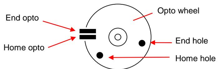
Check the end position as well: move the needle down. Adjustment is successful if end LED goes on before moving part reaches end of mechanical range.
