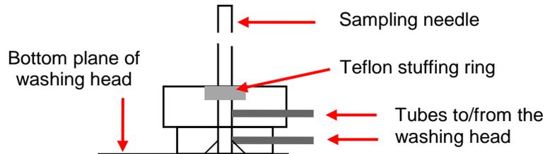
Check the setting of the needle. If end of the needle is at the bottom of the washing head, needle is set correctly. If not, open screws "B" (see above), and adjust the needle to the bottom of the washing head. Fasten "B" screws.
