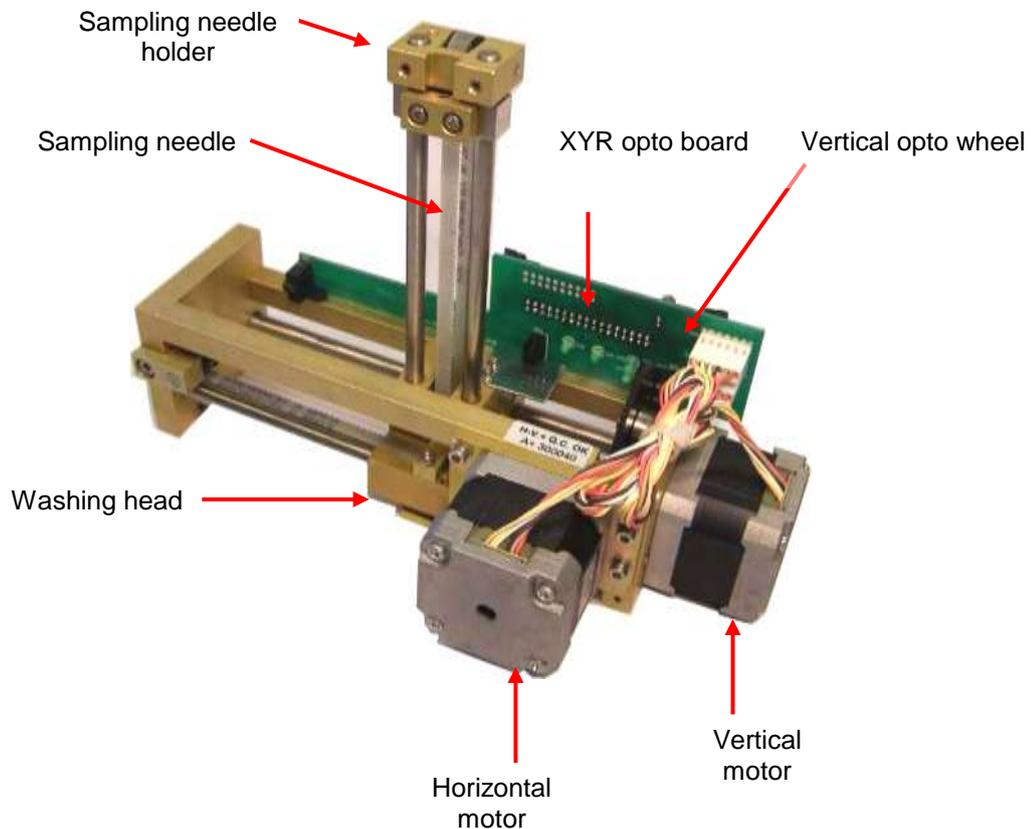
Both stepper motors have optical end-switch sensors for detecting these positions. These are required for correct initialization and error detection. All sensors have status LEDs to show actual conditions.
