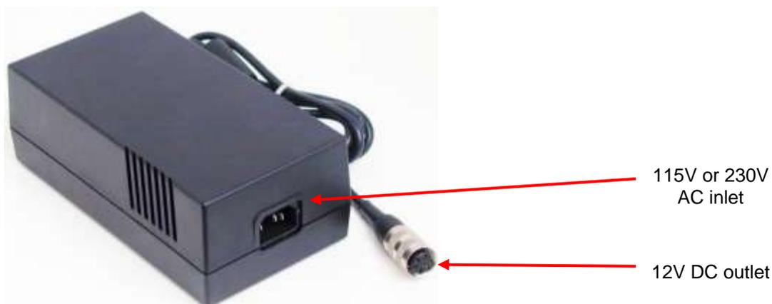
The power supply modules have an auto range input, which makes possible to use them with 230V or 115V mains outlet and it has the CE and UL safety certification. The input socket of the power supply is a standard 3-terminal plug, with power cable connection; the output is a special, lockable socket as it is shown in the picture.
