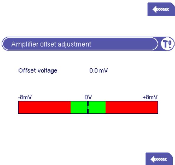
**Offset adjustment:** You can adjust the offset on the amplifier board. The lower indicator (line) represents the measured voltage.
