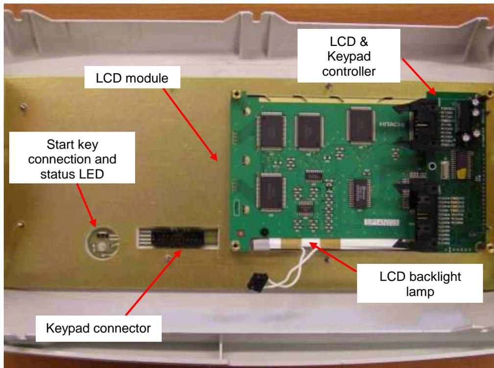
Display assembly contains the 320x240 dots color graphical LCD display and the high voltage board. LCD has a high voltage backlight lamp (high voltage board generates the required voltage).
