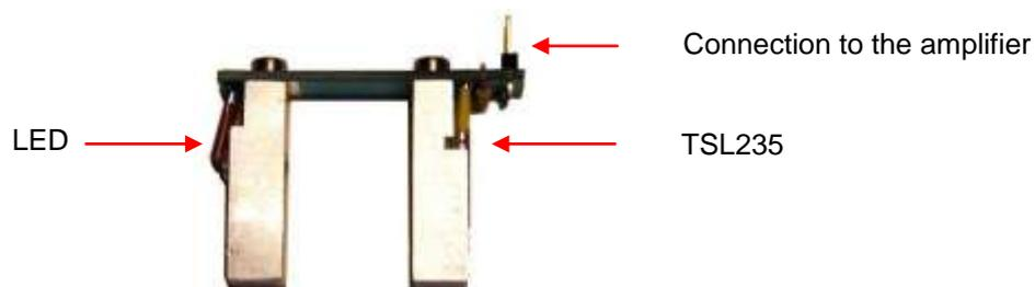
The analyzer performs enhanced Hemoglobin measurement technology for HGB measurement. The output of HGB head is frequency (TSL235 detector is light to frequency converter). This signal is counted by a digital counter in the FPGA circuit/micro-controller.
