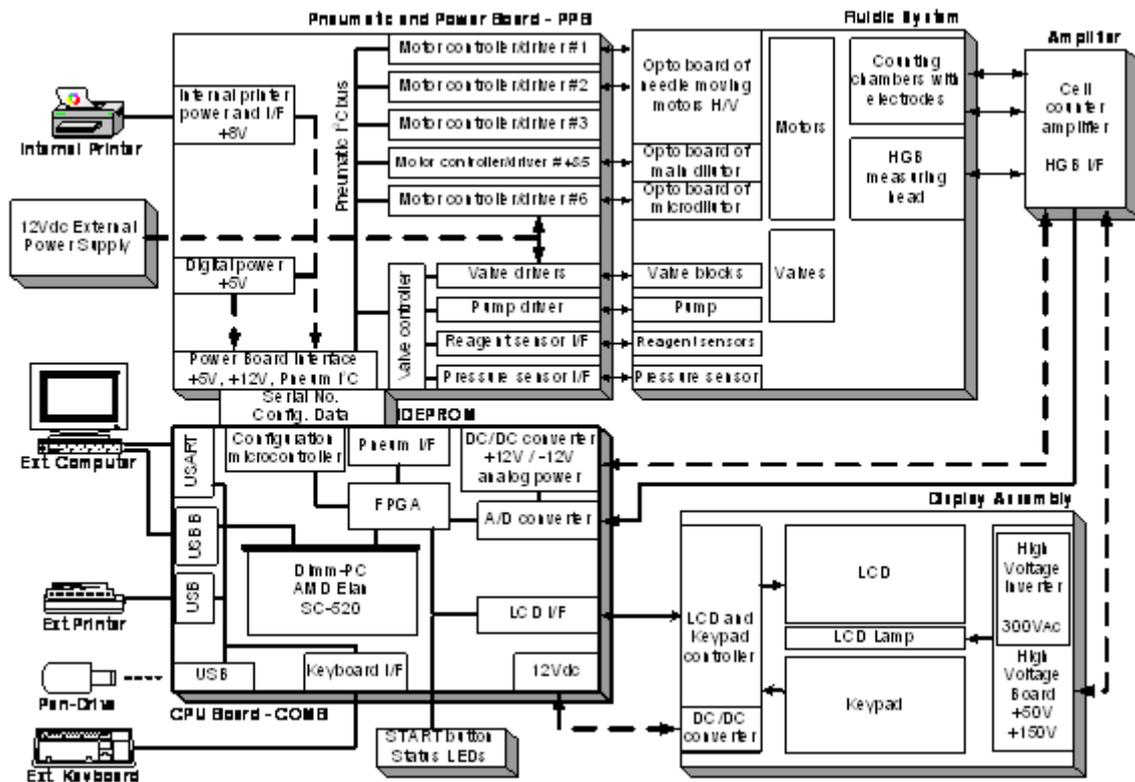
*Hemolyzer 3 Electronic Functional Block Diagram*
