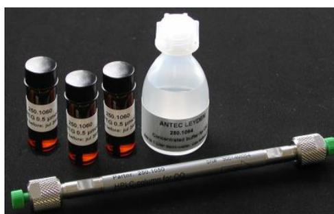
Fig. 1. Part of PQ for HPLC/ECD kit.
