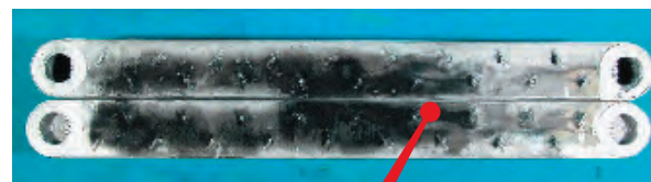
Corrosion occurred on the surface of the oil coolers
