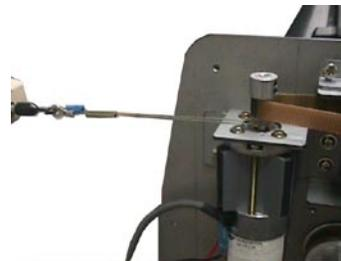
5. Remove the wire/rope from the Y-drive motor.
