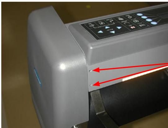
Loosen the two (2) M3 Binder head screws
