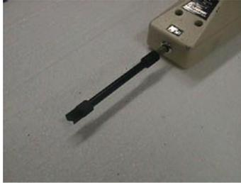
4. Use the force gauge to push the X-drive motor pulley flange with a  $2.25\text{kg} \pm 0.2\text{kg}$  force.
