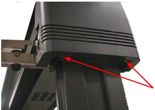
Remove the two (2) M3 SEMS (pan head screw with flat washer) screws
