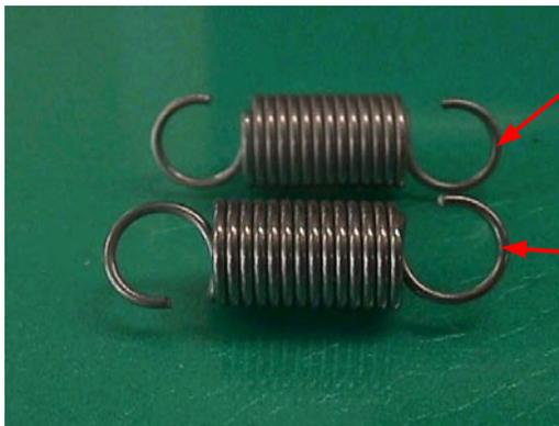
The hooks face the same direction for the left and right pinch roller springs.
