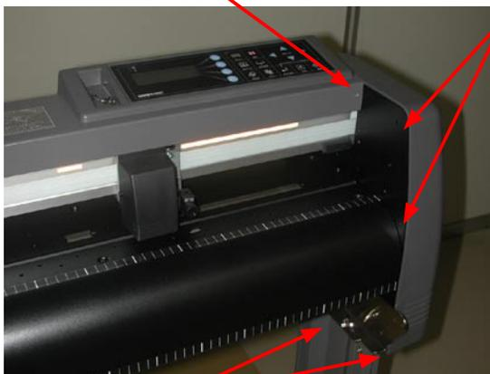
Remove the two (2) black zinc-plated M3 Binder head screws
