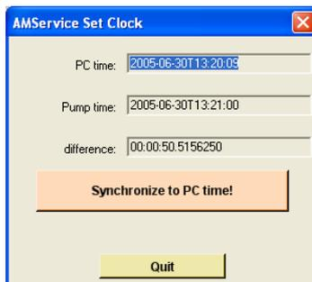
Please note: The pump internal clock will set to the central European time zone (Bern, CET, GMT +1.00h) as ex-works settings, the pump internal clock will not switch automatically between summer and winter time. All history logs (refer to *chapter 4.3.5*) will base on this time.
