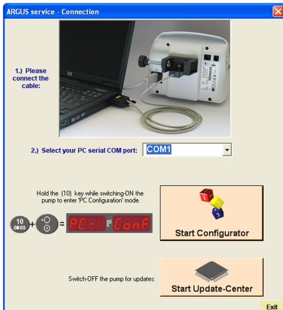
Hold the “10” key while switching-ON the pump.
