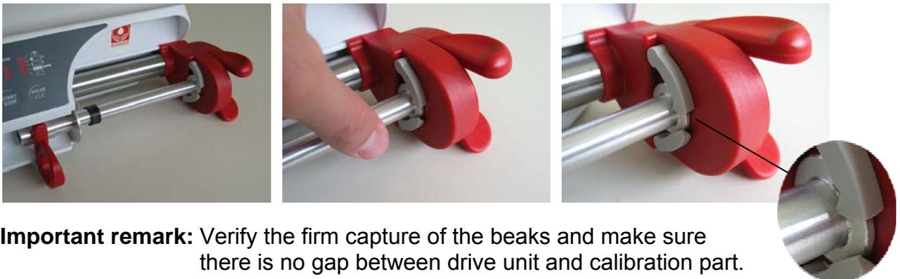
**Important remark:** Verify the firm capture of the beaks and make sure there is no gap between drive unit and calibration part.
