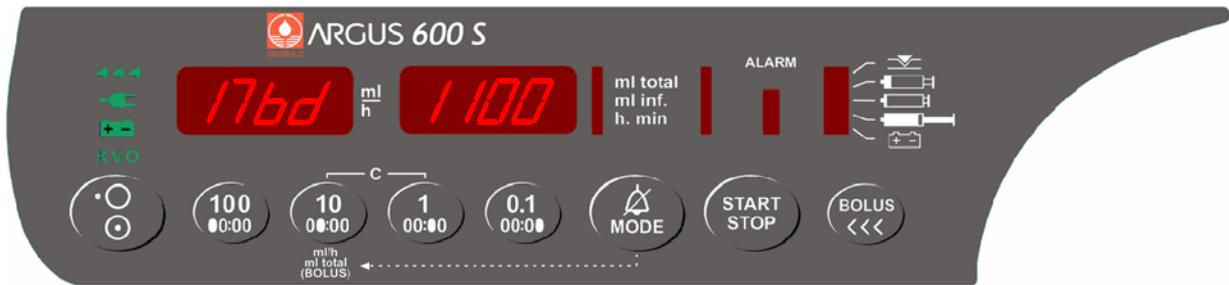
Press “START/STOP” key to store the barrel diameter for 17 mm.
