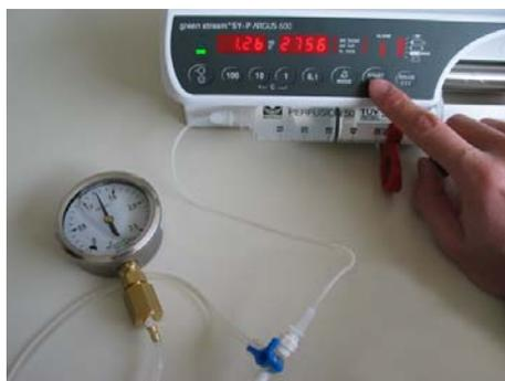
Wait until 1.2 bar is reached on the scale and then press the "START/STOP" key immediately, to register the maximal pressure limit value for 1.2 bar. Switch off the pump.
