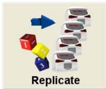
Use this feature to replicate fast and easily pump configuration from a saved configuration file or from a pump to another. A configuration can only be replicated if the saved configuration (and pump type) corresponds with the firmware of the connected pump in the first 2 digits (for e.g. 4.30 to 4.31 is possible).
