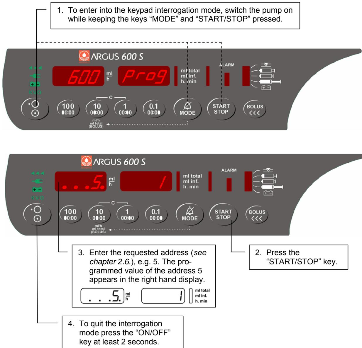
Flashing decimal points indicate which display is ready to accept an input by the keys 100, 10 & 1.
