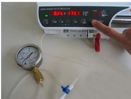
Simulate an occlusion by the 3-way stop cock and start a pressure build-up. Wait until 0.2 bar is reached on the scale and then press the "START/STOP" key immediately, to register the minimal pressure limit value for 0.2 bar.
