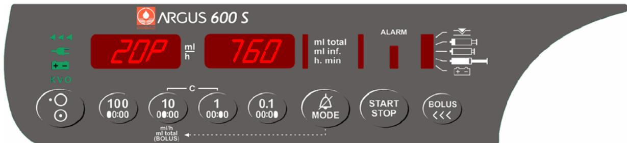
Press "START/STOP" key to store the plunger length for 20 mm.
