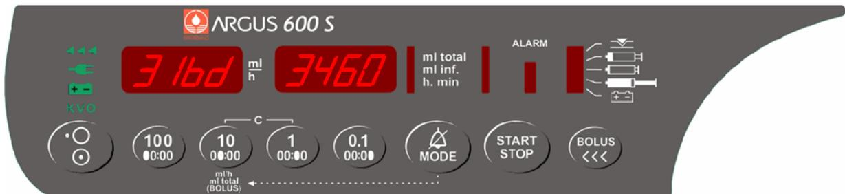
Press "START/STOP" key to store the barrel diameter for 31 mm.
