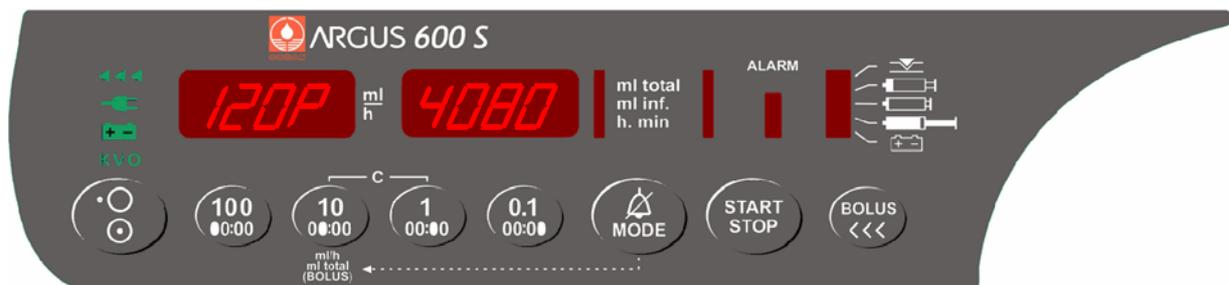
Press “START/STOP” key to store the plunger length for 120 mm.
