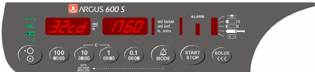
Press "START/STOP" key to store the clamp diameter for 32 mm and then remove the calibration part-1.
