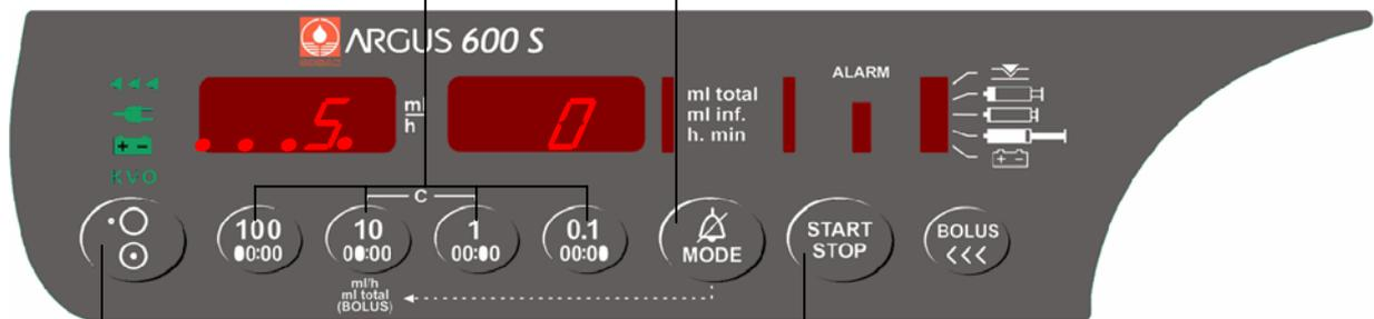
10. To quit the configuration mode press the "ON/OFF" key at least 2 seconds. Changes in configuration become active, after the pump is switched on normally again.
