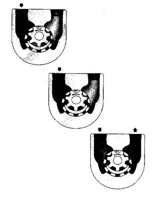
When the teeth mesh on the pressure side, the liquid is forced from the spaces and out through the discharge port.
