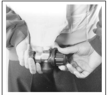
1. Release the handwheel lock and close the cylinder valve. Keep hold of the handwheel.
