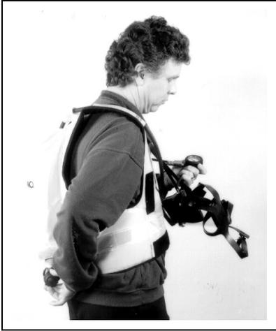
1. Open cylinder valve fully. Check pressure gauge to ensure that the cylinder is at least 80% FULL:
