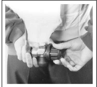
1. Disengage handwheel locking mechanism and close cylinder valve.
