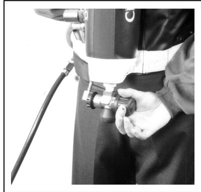
2. Open cylinder valve fully.
