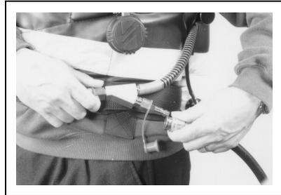
3. Push hose couplings together and pull back collar to release supply hose.
