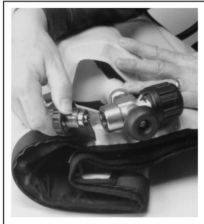
2. Check O-ring on cylinder connector to ensure that it is clean and in good condition.
