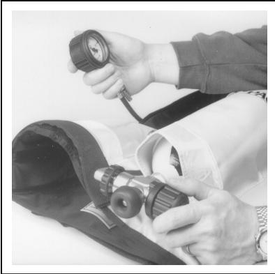
1. Slowly open cylinder valve fully, check pressure gauge to ensure that the cylinder is at least 80% FULL:
