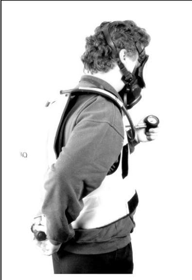
1. Turn the red bypass to ON and check that there is a steady flow of air into the mask. Turn the bypass to OFF.
