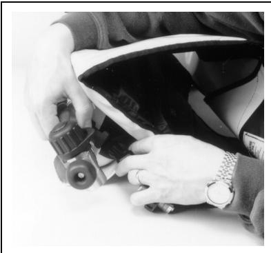
1. Slide fully charged cylinder into pouch and secure using buckle positioned behind cylinder valve i.e. towards the wearer.
