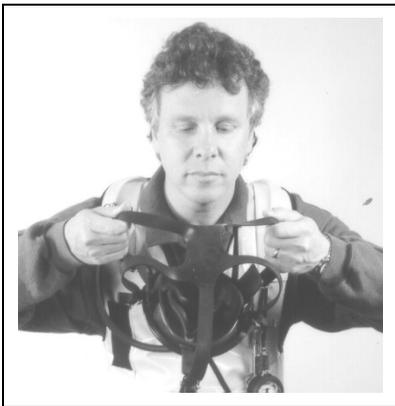
1. With head harness straps fully slackened, place chin into chin-cup and pull harness straps over back of head.
