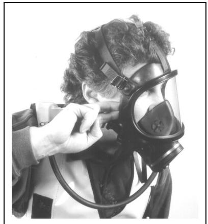
1. Insert finger under face seal and check for a steady outward flow of air. Remove finger and allow mask to re-seal.
