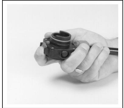
1. Check that orange O-ring on demand valve outlet is clean and in good condition.
