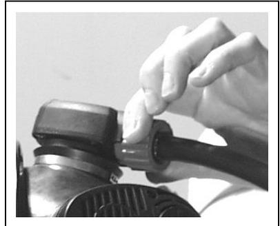
3. Turn red bypass knob to 'ON' position and bleed air from system.
