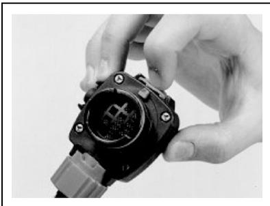
1. Check that the demand valve locking catch is free to move without sticking by depressing the catch a number of times.
