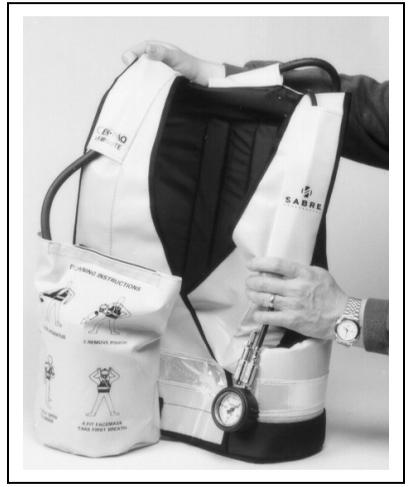
1. Slacken all straps and check apparatus to ensure that it is clean and in good condition.
