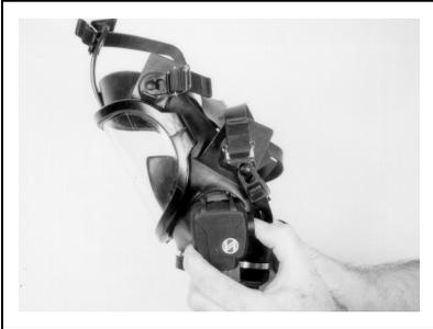
1. Remove facemask from stowage pouch and hang mask from strap around neck.
