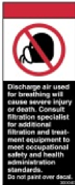
Located on the control panel near air service valve BOSS P/N 300040
