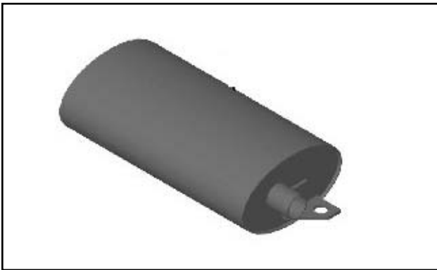
Figure 9 Three way catalytic converter
