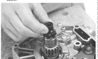
Into a transmission main shaft, put a thrust bearing seat, thrust bearing, thrust washer, and washer in this order, and attach a clutch outer COMP to the transmission main shaft.
