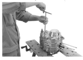
Remove a clutch outer cover, clutch assembly, primary drive gear, clutch center guide and primary driven gear.
