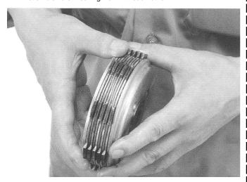
2 . Attach the clutch spacer to the transmission main shaft. Fitting the protrusion on the clutch friction disk into the groove in the clutch outer, and also fitting, at the same time, the spline on the clutch center into the spline on the main shaft, attach the clutch assembly.
