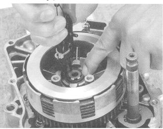
4 . Place four clutch springs into the pressure-plate boss, and fix the clutch lifter plate with a flange bolt. And tighten it to the specified torque diagonally in a few steps.
