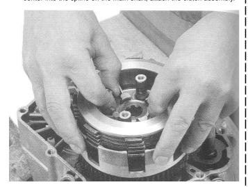
3 .Fit the supplied external circlip to the groove in the main shaft with the circlip's round corner on the downside.
