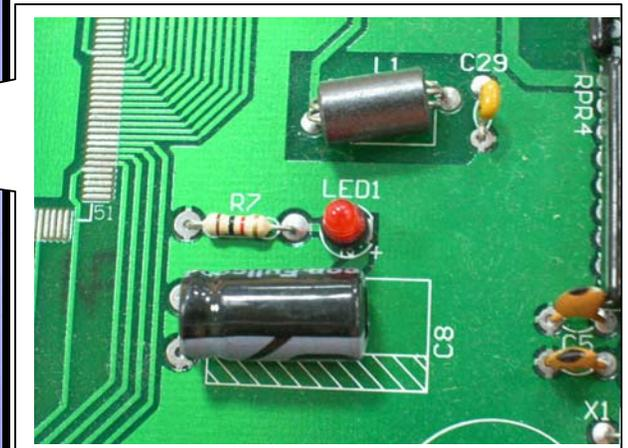
If the display board has power, display VCC LED1 (805p) OR LED13 (807P) indicator (shown above) should light; capacitor C8 (shown above, 805P) should also have power. To test voltage at the capacitor, put a multimeter probe on each pin of capacitor C8. Normal reading: 5 VDC. If there is power at the display but it doesn't light or beep once when turned on, replace the display. If there is no power at the display, make sure the ribbon cable is connected well and inspect the drive board.
