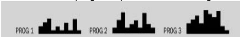
Illustration height represents resistance: the higher the column, the more resistance. (One dot (below) represents two resistance levels.) Horizontal length represents time. Once in exercise program mode, the main window shows a picture like the one below.
