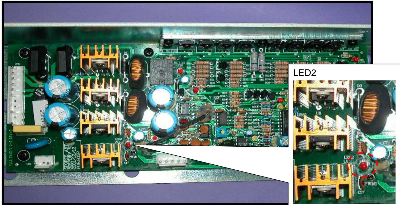
If there is power to the drive board, the drive board VCC LED2 should light. If not, inspect the transformer input and output voltages, fuse, fuse holder, and on/off switch.
