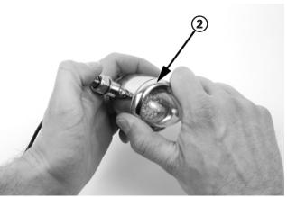
With the lens cover (2) off, you can remove the gasket (4) and swap the lens (3). Replace the gasket and press the lens cover back onto the lamp's main body (5) and rotate it COUNTER-CLOCKWISE 90-degress to lock it into place. Once you have completed the lens charge or cover reorientation, reinstall the retention screw.
