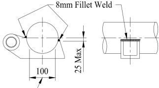
No welding on the bottom half of the axle tube. This includes positioning tack welds.
