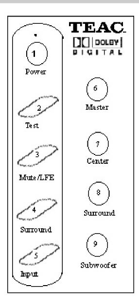
another. During the test the corresponding LEDs at the front panel of the decoder unit light and show which of the speakers the test signal is actually applied (/L, /C, /R, /SR, /SL, /LFE). After passing the test the system resumes with the last settings.
