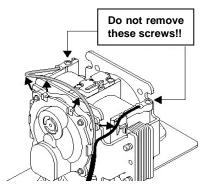
3. Remove a power cable from 4 hooks. **Do not remove** screws!!
