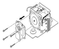
4. Remove 4 screws from a casing.
