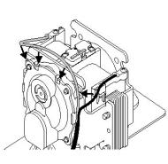
8. Fit power cable into 4 hooks.
