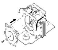
6. Install new diaphragm using new Nylon nut provided. \*Tightening torque – about 1 Nm
