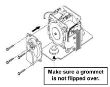
Insert casing air outlet into rubber grommet. Secure with 4 screws.
