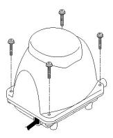
1. Unplug blower. Remove cover bolts using an 8mm-box
