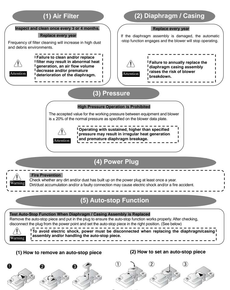
Face ▲symbol from auto-stop piece towards Remove auto-stop ▲symbol on auto stop piece from blower holder and slide the piece into the holder.
