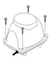
10. Affix cover bolts using an 8mm-box wrench or screwdriver.
