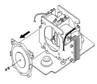
5. Remove Nylon nut and remove diaphragm from body.
