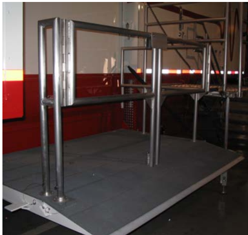
Lift with Hand Rails
