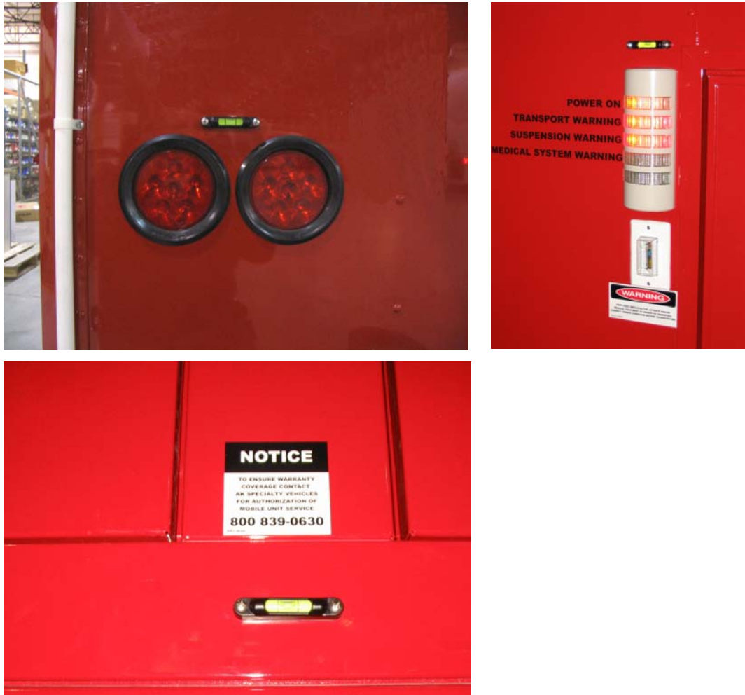
Figure 5: Mobile Unit Spirit Levels
