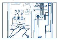
15. To clear the feeding and flush volume delivered, turn dial to CLEAR VOL. (This occurs after four beeps.) NOTE: If alarm sounds, turn pump dial to HOLD. Correct alarm condi-
