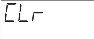
Screen flashes four times at 1 second intervals while CLEAR button is pressed and then Last Flow Rate is displayed
