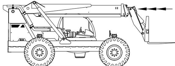
Always place the load in the center and completely against the back of the fork frame. By doing so greater stability will result.
