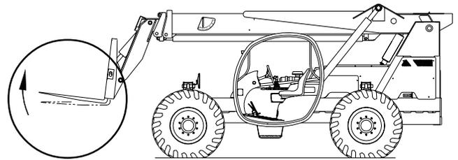
The load should be kept as low to the ground as possible while traveling. Always move a loaded machine with the boom angle indicator (D) at 0 degrees or less.
