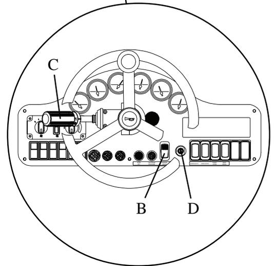
Insert the ignition key in the ignition switch (D). Rotate the key clockwise until the engine starts. Release the key when the engine starts.
