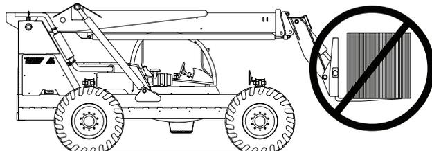
**IMPORTANT:** Never attempt to use the forks and/or attachments for prying wedged or frozen loads free. Damage to the load, pallet and/or machine could result.
