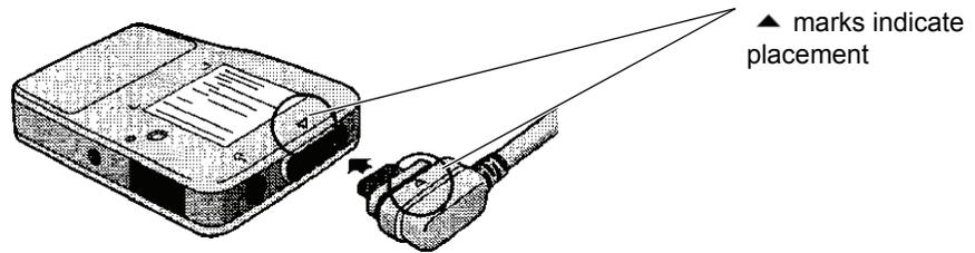
Connect the patient cable to the connector of the recorder with the ▲ mark facing up. Make sure it is connected properly.
