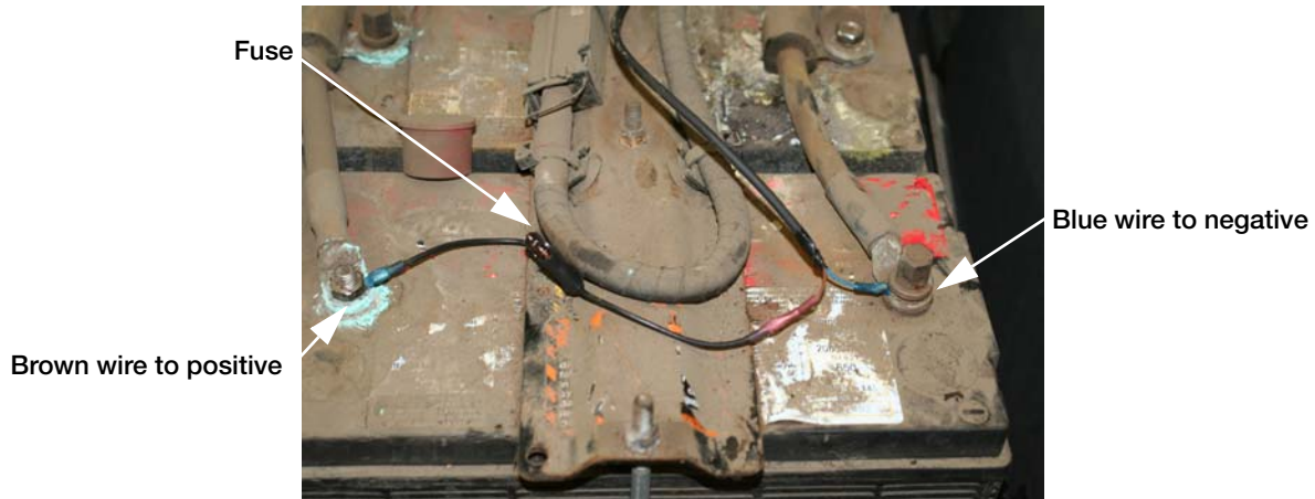
Figure 3-5. Power Connection to Battery
