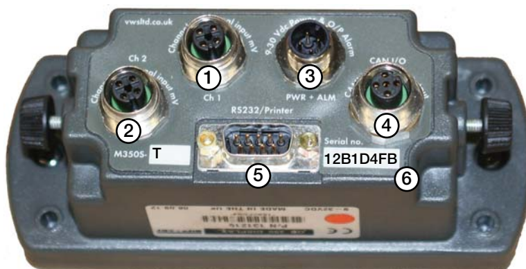
Figure 3-10. Rear Panel Identification and Bulkhead Connectors
