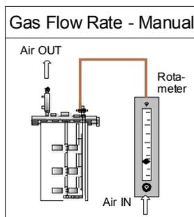
Unless specified otherwise, control of gas flow into the fermenter is usually set manually. A separate pump or laboratory air supply is connected to the fermenter supply pipework which has an integral pressure regulator valve. The flow rate is adjusted using a rotameter calibrated in litres per minute/hour. The maximum air flow rate should be no more than 1.5 vessel volumes per minute. A mass flow valve and/or gas mixing system may also be used.
