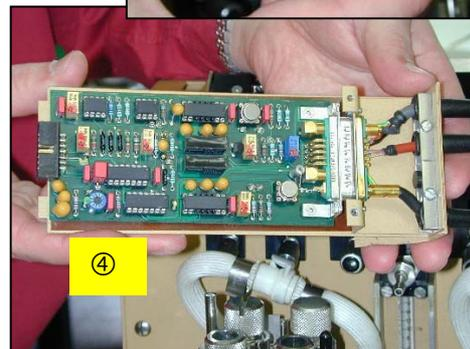
Measurement module with operational amplifiers pcb
