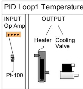
Temperature is controlled using an electrical heating block with in-built cooling coil. The range of control is approximately 5°C above the cooling temperature to 60°C. A signal from a Pt-100 temperature sensor in the culture is used for feedback control by the micro-processor to activate either the heater or the cooling valve. The main controller display shows actual value, setpoint PID control etc.
