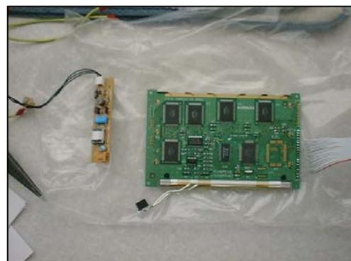
LCD Screen & Light/Buzzer pcb (18335) removed
