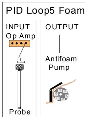
Control of foam is based on a conductivity probe above the culture surface detecting the build-up of foam by contact with the probe tip. The rest of the probe is insulated to prevent false signals. After a user-selectable waiting time (delay) the integral peristaltic pump delivers a dose of antifoam reagent (shot). The system then resets and will only add more reagent if foam is still present. This arrangement can double as a level control system to remove culture.
