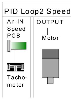
A setpoint is given to the control circuitry by the microprocessor. The PID control values are factory set for this parameter. The main display shows the actual value for speed. The level of dissolved oxygen can be cascaded to influence the stirrer speed. Speed range is typically 20-1200 rpm upper and lower limits depending on the EPROM installed for a specific application. No service adjustments can be made.
