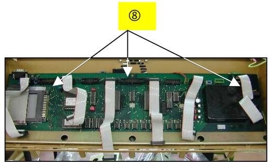
Replacing main pcb
