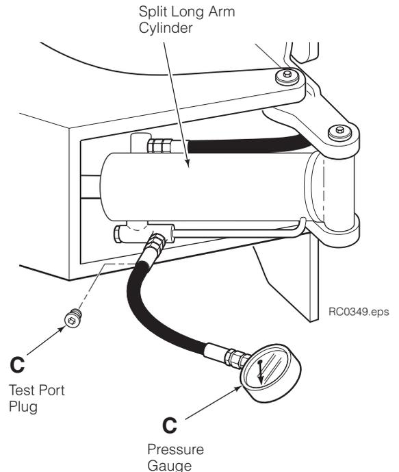
**IMPORTANT:** If truck is equipped with a 3 or 4 pressure selection valve, adjust split arm relief cartridges while pressure selection valve is at its lowest supply setting.
